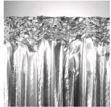
Figure 6. Honeycomb crushed in the direction of the cell axis
