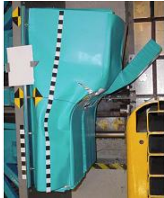
b) Half Wall test (top view)
